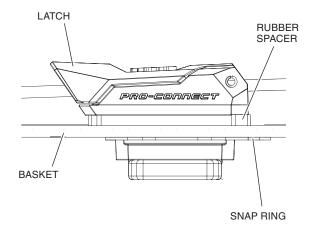
3. Lift the lever on each latch to unlock them. Place the utility basket onto the front rack of the ATV. Line up each latch with its corresponding hole in the rack then push each latch into its hole.
