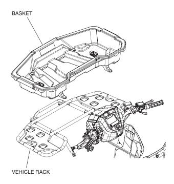
Secure the utility basket to the mounting plate by pressing down each Honda Pro-Connect<sup>™</sup> lever.
